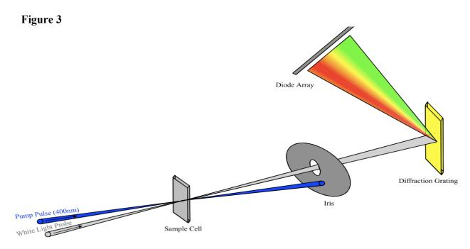
Notes: Schematic of pump-probe spectroscopy.
