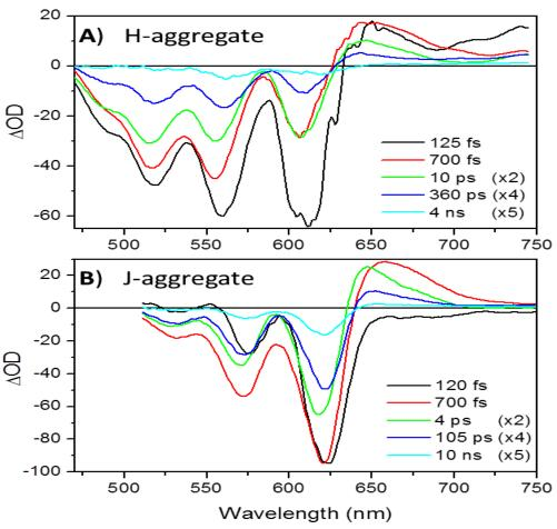
Notes: EADS of A) P3HT H-aggregate and B) P3HT J-aggregate. Each EADS spectrum represents the state of the polymer at the associated timescale.
