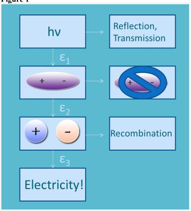
Notes: Flowchart demonstrating how the efficiency of each process can dictate the overall efficiency. The formations of the second and third boxes on the left side, which represent polaron pairs and delocalized polarons respectively, occur on ultrafast timescales that can be resolved with ultrafast laser spectroscopy.
