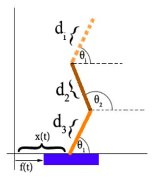
Figure 1: An arbitrary *n*-Link inverted pendulum system
